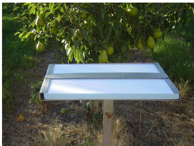
Figure 2. (a) Hailpad used in the ADV-TP. Source: M. Torà. (b) Plate with impacts painted in black, prepared for analysis. The central strip presents the impacts done in laboratory to do the calibration. Source: Atmospheric Physics Group, Universidad de León .
