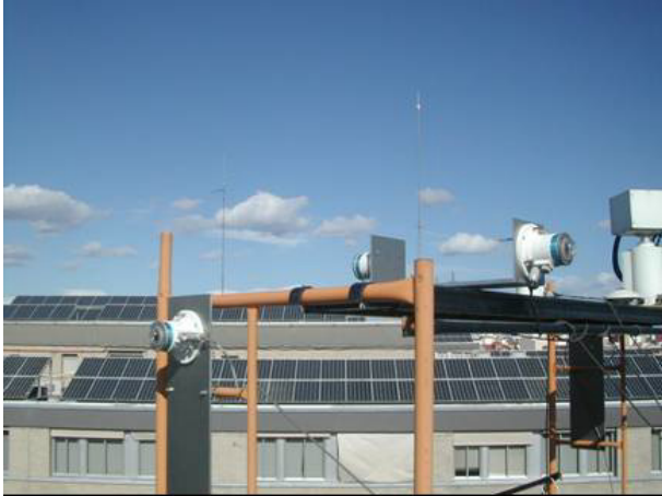
Figure 1. Experimental device for the measurement of ultraviolet erythemal radiation (UVER) on vertical planes (partial view).
